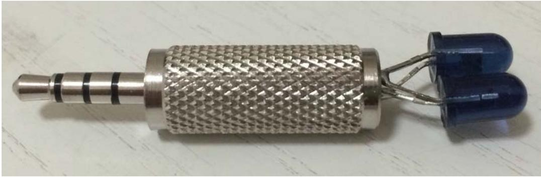
**This is the emitter which is used to connect with smartphones and produce infrared signal.**
