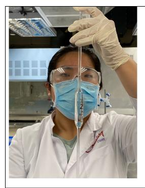
I am dressed in lab-appropriate attire and using a volumetric pipette to measure out 25.00 milliliters of solution.
